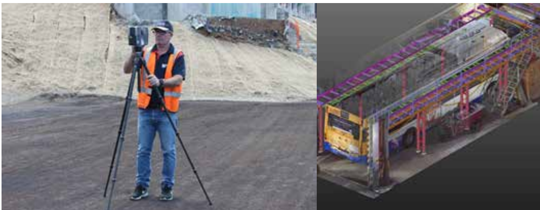
A Watkins Steel staff member in the field with a 3D scanner (left) and an image of an area of the Toowong Bus Depot. Photos courtesy of Watkins Steel.
